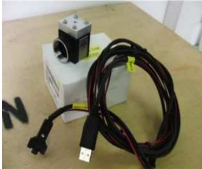
P32.7 2-Camera CMOS Monochrome IDS-UI 1240SE-M
