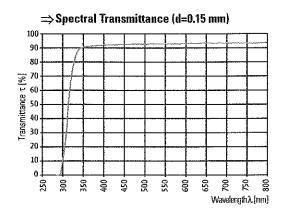
The light transmittance for a thickness of 0.15 mm is types in %  $(d=0.15 \text{ mm}) = 91.7 \pm 0.3\%$ . In the visible range of the spectrum D 263 M is without absorption. The excellent UV absorption properties make D 263 M an ideal material for use in fluorescence microscopy.
