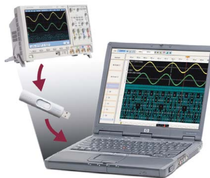
Figure 13. View and analyze previously acquired scope data on a PC-based offline tool
