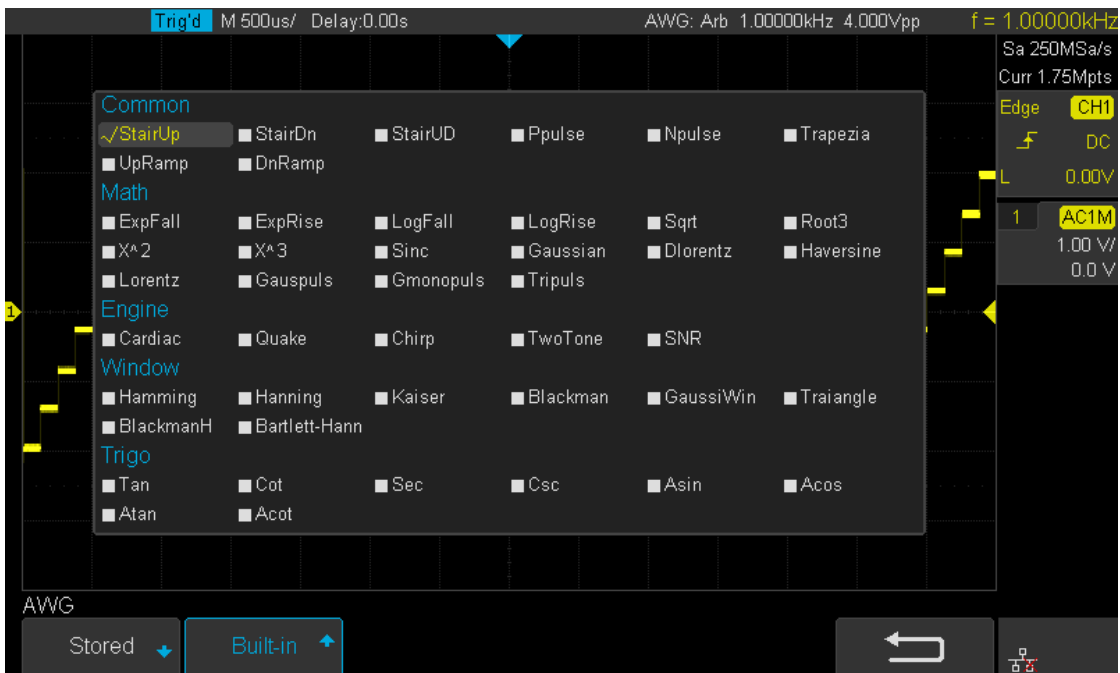
Figure 91 Built_in Arb interface
