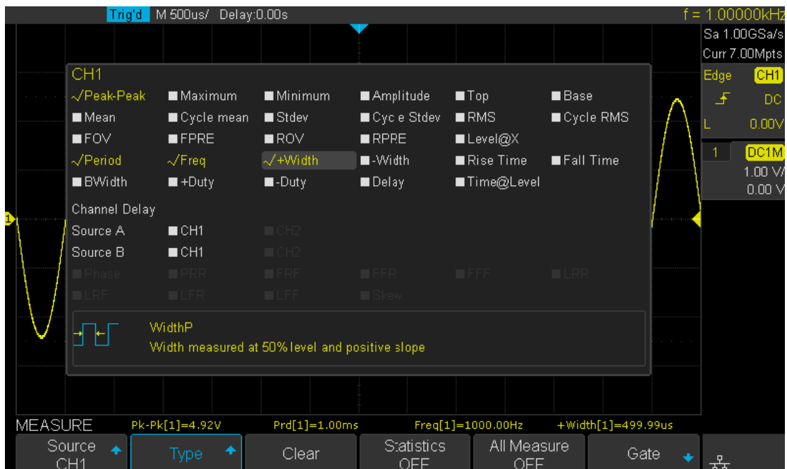
Figure 69 Select the Measurement Parameter
