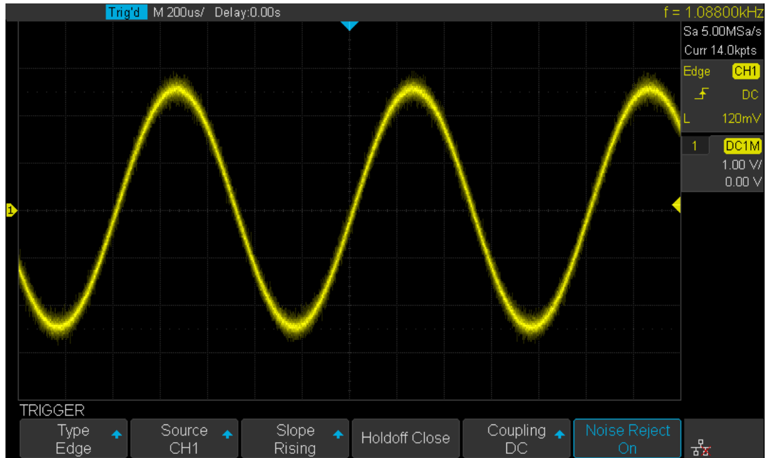
Figure 26 Turn on the Noise Reject
