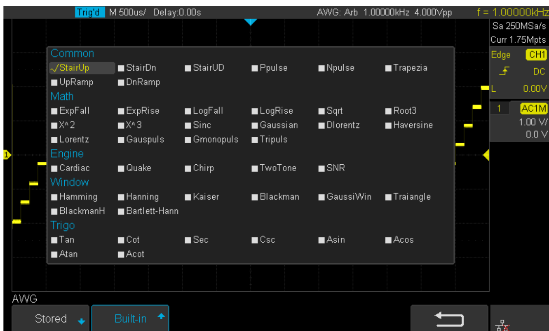
Figure 91 Built_in Arb interface
