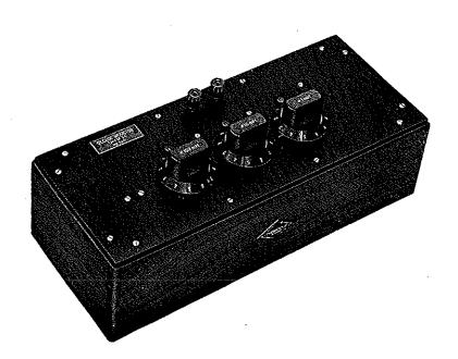
A variable inductor for use as a secondary standard of inductance. The coils are air-cored wound on wooden formers and carefully impregnated and aged for maximum stability.
