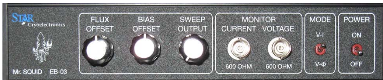
Figure 3-2 Front panel of the Mr. SQUID ® electronic control box.
