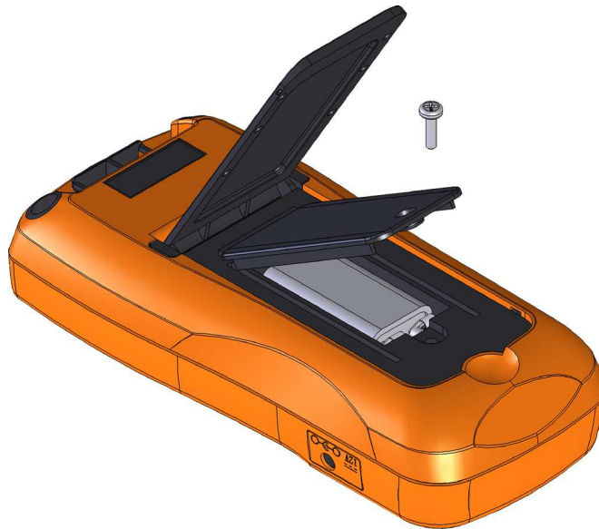
Figure 1-1 Installation des piles
