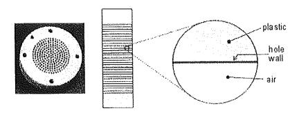
Temperature of the wall changes along the hole. The right end of the plastic part is warmer than the left one because the right end is joined with the copper part of the pipe we hold in our hand while the left end is joined with the copper part cooled in liquid nitrogen. We shall assume that the temperature of the plastic wall rises linearly to the right.
