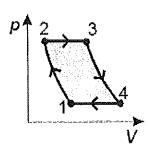
The thermodynamic cycle of the parcel is described with two adiabatic curves (1-2 and 3-4) and two isobaric curves (2-3 and 4-1). The area the cycle encloses in the pressure-volume diagram equals the work released in the cycle. In our case the work is done on the parcel.
