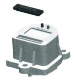
1. Remove the battery / housing cover.
